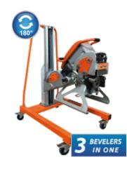
3D adaptive system compensates for the unevenness of the floor and enables positioning of the machine according to the situation at the workplace.
